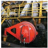
With its extreme torque-toweight ratio and compact design, the Hägglunds CBM hydraulic direct drive is able to handle a very broad range of tasks in rugged operating environments.
