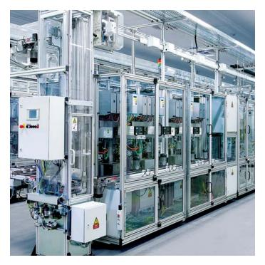
Rexroth's aluminum structural framing provides the flexible and versatile core of our ergonomic Manual Production System workstations. Featuring easily reconfigurable material transport components, flow racks and a complete range of bolt-together workstation elements, they provide the perfect platform for lean, demand-driven assembly solutions.
