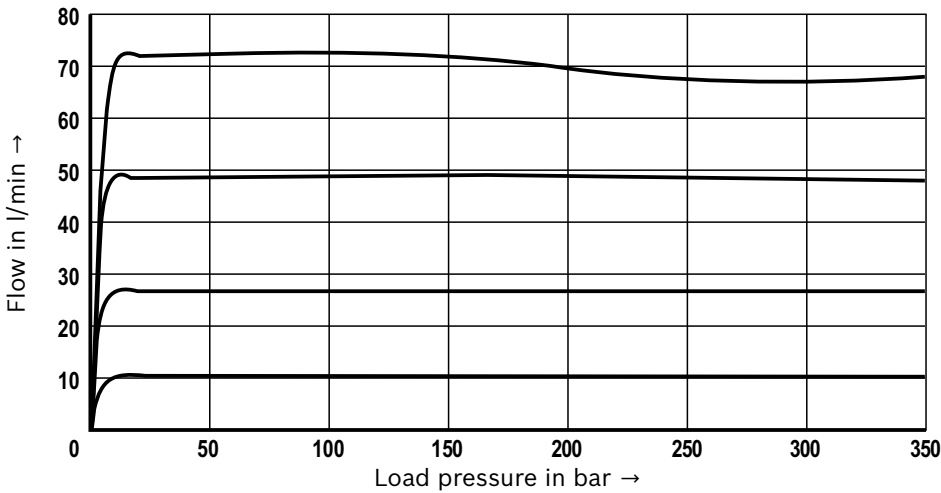
Regulated flow at main port ③ as a function of the load pressure 2-way function (main port ② closed)
